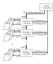
Fig. 1. A 256  $\times$  256 scalable scheduling architecture using 8  $32\times256$  scheduling devices.
