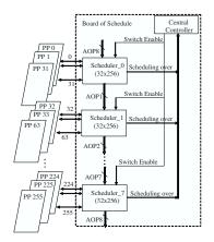
Fig. 4. The architecture of distributed parallel scheduling.
